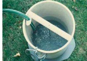
Bench testing offers accuracy and volume controls that can't be obtained in the field. Field testing (using bib cocks, volumetric buckets, or garden hose/test meter) may offer speed advantages, but there are factors
