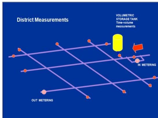
Historically it has been shown that the 80:20 rule holds true when reviewing leak detection and line break trends. In other words 80% of the problems are usually found in 20% of the pipe network. The concept of district measurements (recent
